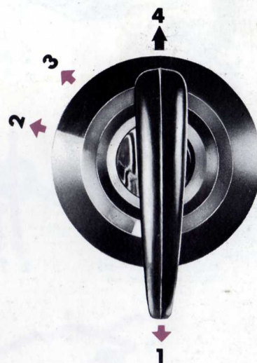
Fig. 13 b - Anti-theft device 1 - Anti-theft position 2 - Garage position 3 - Ignition 4 - Starter
