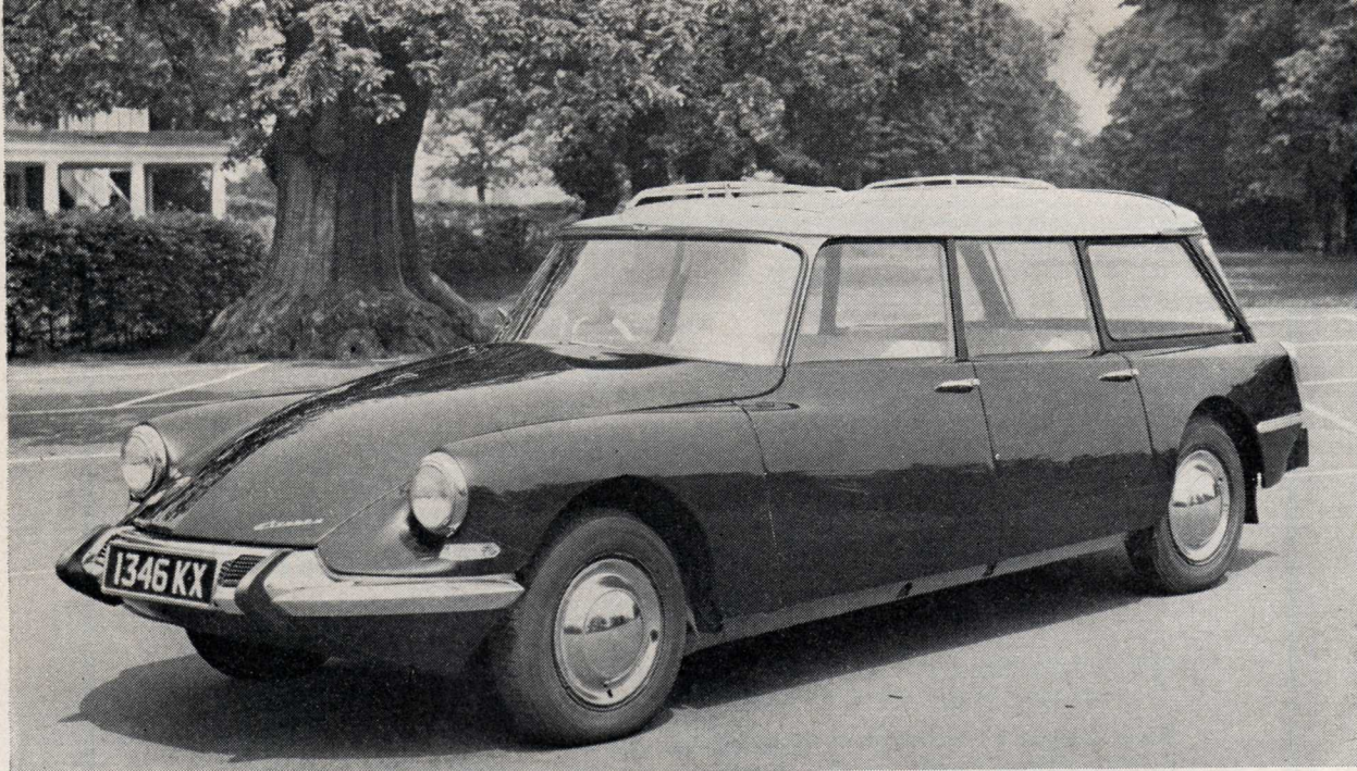
The Safari is an impressive and purposeful looking car. Rubber overriders protect a projecting front which houses the spare wheel, tools, gearbox and radiator, the last having a ducted feed from a low air intake.
